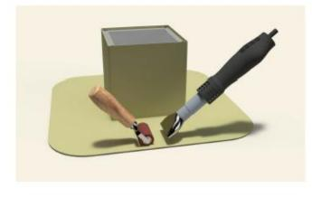
Step 10: Drop down the TPO boot over the roof curb.
